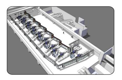
The station was constructed under an existing portion of Concourse B. The A-Gates Station is operating in a center platform configuration. Passengers arrive at and leave the Station from a single platform. It will eventually be expanded into a side/center/side configuration. Several of the former B-Gates were re-designated as A-Gates to reflect their proximity to this station.
